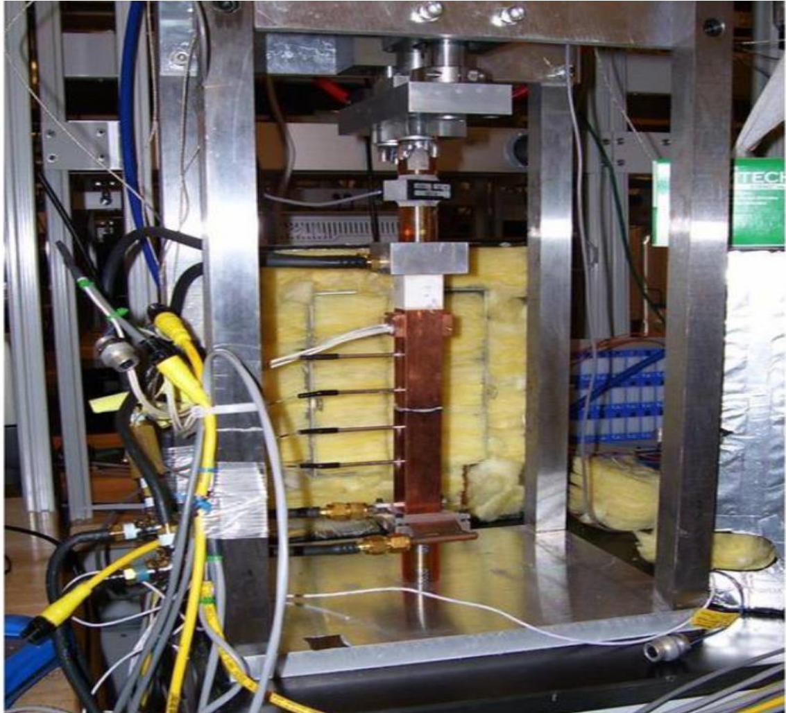
Figure 5-5 Schematic of steady state method setup, where an electric power provides heat from the top of the setup, and an oil bath at the bottom functions as the cooling system, thus generating a steady temperature gradient. Four thermocouples are used to detect the temperature located at certain places of the copper rods, and an insulator box is added to reduce the heat loss during the measurements.
